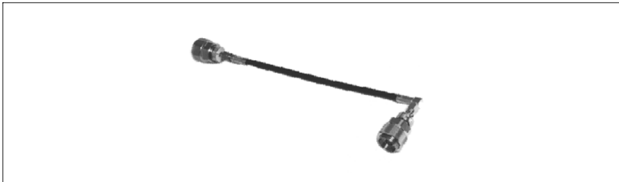
Figure 83 Photograph of DUT No. 1 with SMA connectors and the test port adaptors (SMA-PC7)
