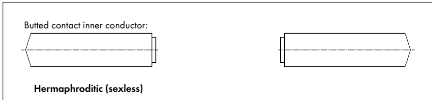
Figure 43 Butted contact inner conductor
